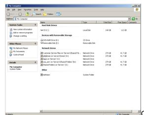
making sure the micro SD card is inserted and the VOX switch is off, turn the device on. The device will show up under Devices with Removable Storage and will be assigned the next available Drive letter. In the above screen shot, the next available drive letter was "e" so that is the drive letter assigned.
