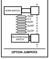
**Two-Tone** - Two-Tone can replace Thunder by cutting the resistor jumper labeled "T-T". **Thunder/Horn Disable** - Some jurisdictions do not allow special tones in the siren. The Thunder and Horn functions can be completely disabled by cutting the resistor jumper labeled "TH/H".
