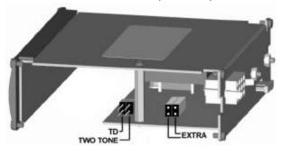
**Thunder Disable** - The Thunder function can be comp letely disabled by moving one of the option jumpers inside the amplifier unit from "Extra" to the "TD". When Thunder is disabled, the Manual button will not have any effect on the tone while the siren is in the Yelp mode
