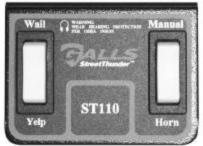
**Center Off** – (Manual/Standby) - A silent mode that allows momentary pushbutton Manual and momentary push-button Horn. The siren output *winds down* when the Manual momentary switch is released.
