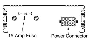
connector before installing the connector on the unit. If the unit needs service, the power connector can be easily removed without unwiring the connector.
